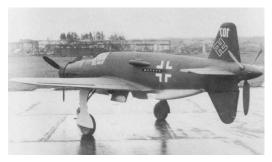
(May): **Dornier Do 335** (Left): The unique pushpull engine configuration of the "Do 335" had been patented by Dr. Claude Dornier in 1937, but a prototype warplane did not fly until 1943. Performance was exceptional but delays and diversification into night-fighter and
